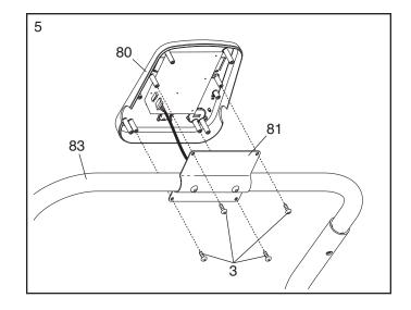
Attach the console back to the Console (80) with the four M4.2 x 12mm Screws (3) that you removed in step 4.
